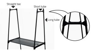
Take 4 long pipes, 4 straight tees, 2 short pipes, and assemble as shown in the figure
