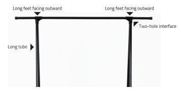
Take 5 long tube and 2 double-hole interfaces, assembling as shown in the picture
